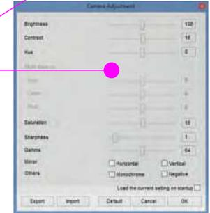
Camera adjustment settings such as white balance, auto exposure, etc.
