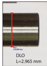
Application with Dino-Lite USB Microscope with edge detection. For Dino-Lite microscopes, see our catalog.
